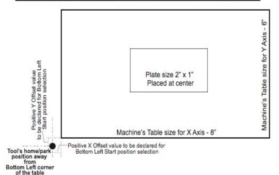
Tool is parked at the Bottom Left and away from the table(machine) and home position should be Bottom Left. Following choise is available for Start position and respective offset values to enter:
