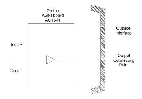
The controller is equipped with output line drivers IC's ACT541.
