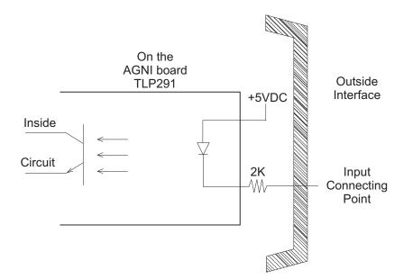
All the inputs are optically isolated with a 2K resistor to limit the current flowing through the diode. Each of the inputs is equipped with the above circuit.
