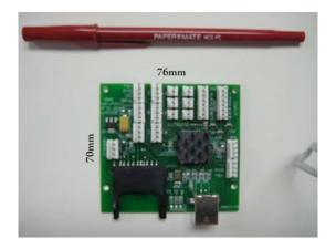
The USB controller board with necessary connectors, USB cable, and SD memory card
