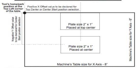
Tool is parked at the Top Left corner of the table(machine) and home position selection should be Top Left. Following three choises are available for Start position and respective offset values to enter:
