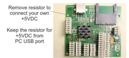
Version II USB controller shipped from 2008. Positions for Motor Output connections for A, X, and Y has been changed compared to version I. Similarly positions for Output connectors B, D, and F also has changed.
