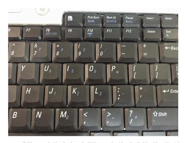
These keys are available to use in NumLock mode. Either pressing Num Lock (NumLk or Num) key by itself or using the shift key + Num Lock key brings that numeric mode. The Numeric mode also can be confirmed in most computers by a display of a light with a lock symbol and number '9" in it. Now, to use these numeric keys user will have to press Fn key along with any one of the numeric keys. Fn key is located on the left side of the keyboard near the Ctrl and Alt keys.
