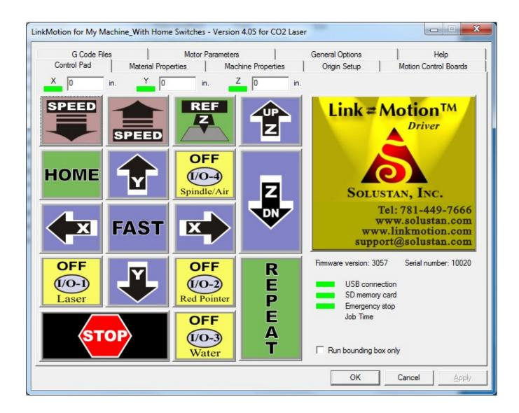
The Control Pad is operated using the numeric keypad on the right side of the extended PC keyboard. The screen design of the Control Pad mimics the actual numeric keypad. This is the main user interface for the LinkMotion driver software on the PC. Besides controlling the movement of the machine using the Control Pad, it supports many different tabs for to customizing LinkMotion machine settings.
